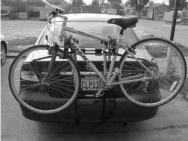
Fig. 6: On a bike with a slanted top tube, place top tube on rear cradle, and down tube on front cradle to keep bike as "level" as possible. For "ladies" style and non-conventional frames, it may not be possible to keep bike "level".
